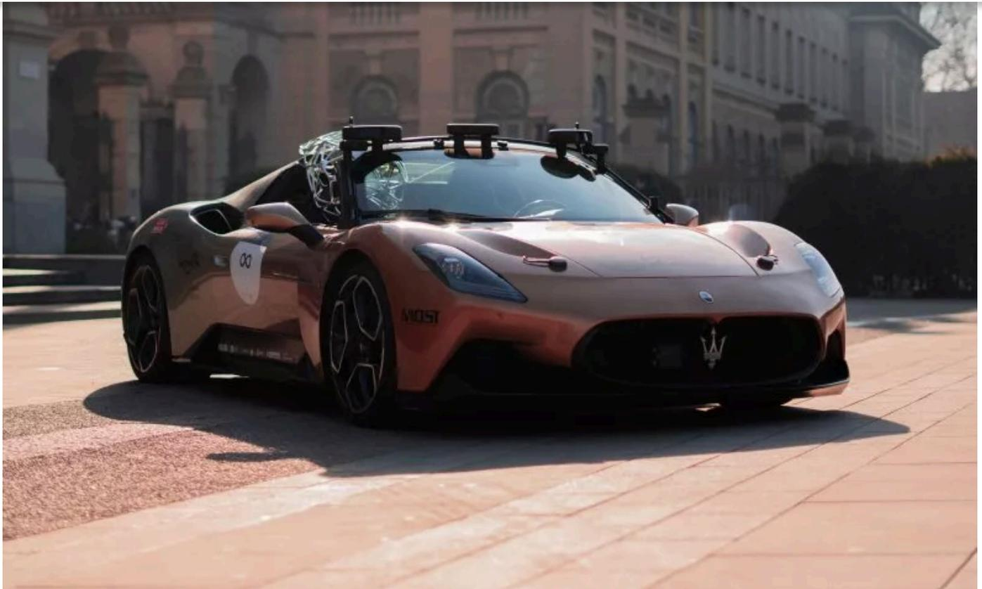
AI-driven Maserati MC20 front view. The special MC20 features radar, LIDAR, sensors and cameras.
